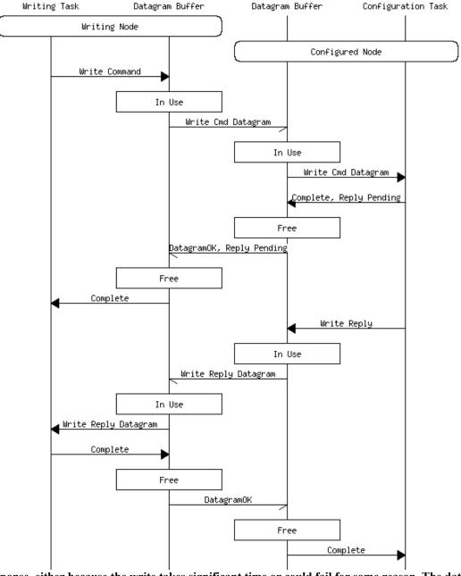
A delayed response, either because the write takes significant time or could fail for some reason. The datagram reply to the Write Command carries the reply pending bit set, and a reply datagram is send from the configured node back to the configuring node with the reply.
