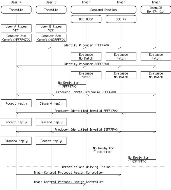
Depending on the packet queuing behavior of the individual Nodes in this interaction the exact sequence might be slightly different. On CAN-bus, the Producer Identified replies have a higher priority than any potential additional request that might be coming in; as such, the replies for the first request will typically precede the second incoming request on the bus. This ensures that Train Nodes and Command Stations do not need an unbounded amount of buffer to handle Train Search Protocol.
